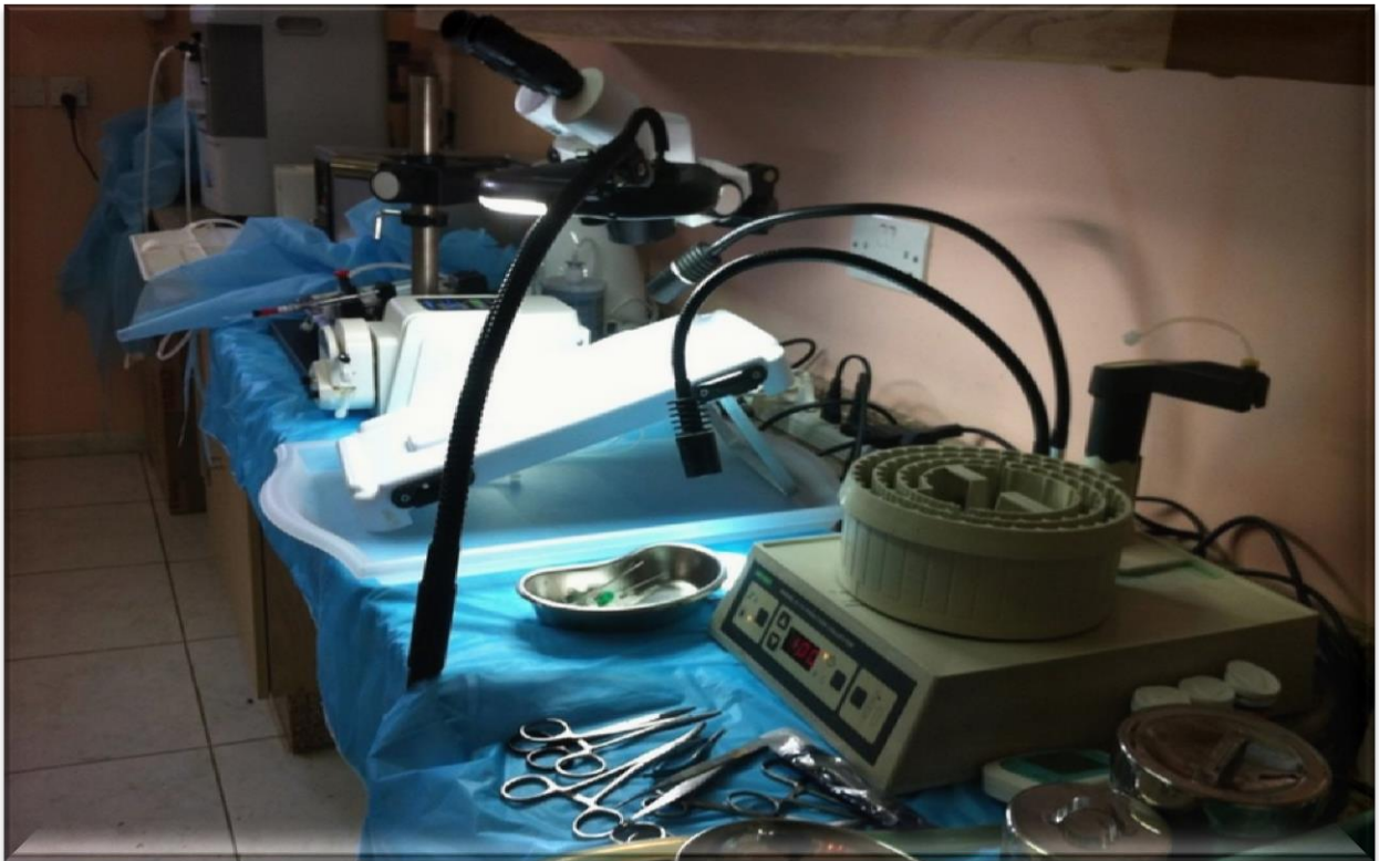
Figure 2.1 Anesthesia system linked to an oxygen concentrator and a peristaltic perfusion pump.
